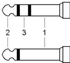
Socket to connect a footswitch, with controlled *Channel* switching and *Gain* selecting. TRS Jack socket (T - tip: 1, R - ring: 2, S - sleeve: 3), where
