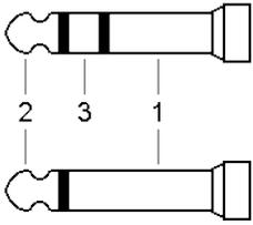
The additional footswitch socket is in TRS form (T – tip: 1; R – ring: 2; S – Sleeve: 3), where the tip activates the bypass of the effects loop, the ring turns the reverb off, and the sleeve is ground.
