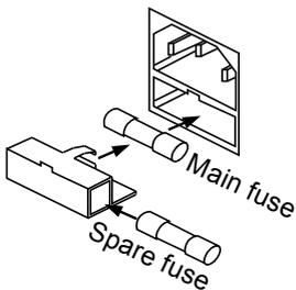
Slo Blo fuse T1.6A is in the case, integrated with power supply socket. There is one spare fuse inside.
