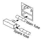
Slo-Blo fuse T1,25A is in the case, integrated with power supply socket. There is one spare fuse included.
