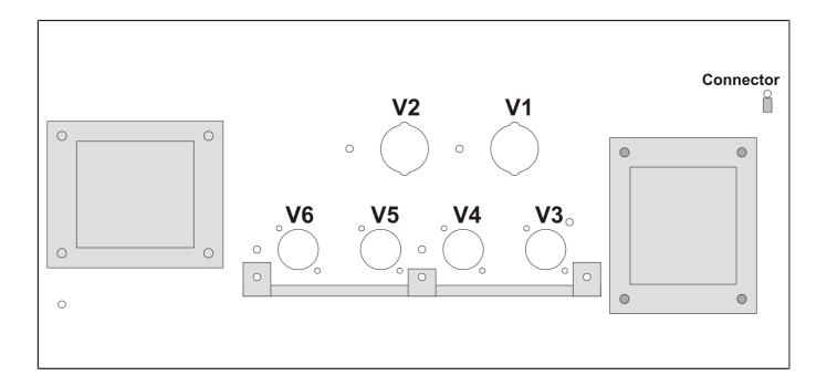
Tube placement in the chassis
