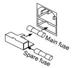
Slo Blo fuse T1.6A is in the case, integrated with power supply socket. There is one spare fuse inside.
